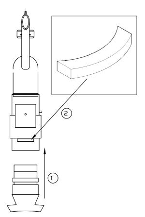
3. Insert Swivel Boss of Dryer or Processor into Pivot Hood [1], lining up the groove in the Boss with the slot in the Hood and place the Locking Wedge in position [2].
