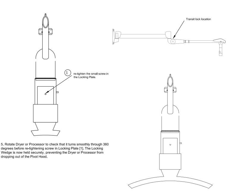
6. Once the Dryer or Processor is in position it is safe to remove the Transit Lock. To accomplish this, gently pull down the Lower Arm (front section) until there is no pressure on the Transit Lock, thus enabling easy removal. (Always keep Transit Lock in a safe place for future use. NEVER REMOVE the Dryer or Processor from the Arm, without first TURNING OFF THE POWER and re-locating the Transit Lock.)
