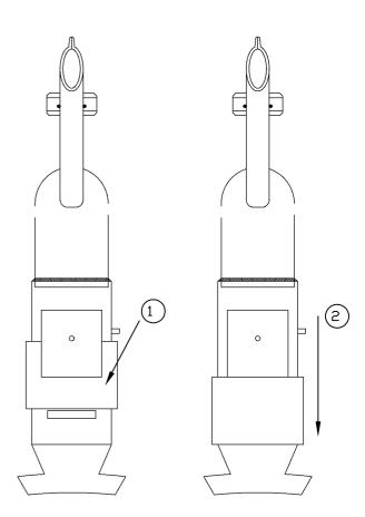
4. Let go of Locking Collar [1] allowing it to fall into place over the Locking Wedge [2].
