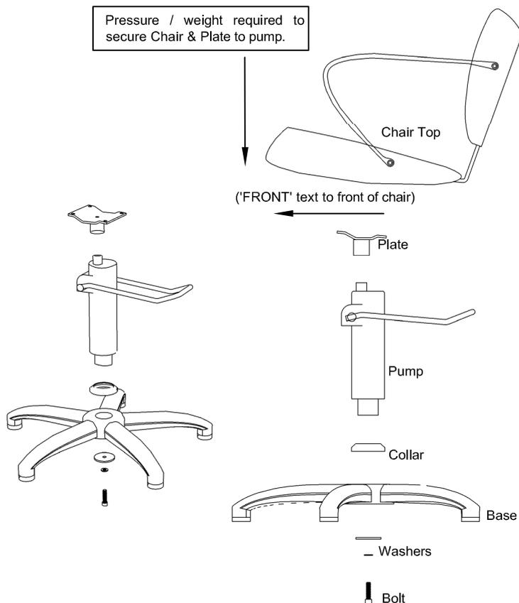
**Ensure the pump pedal is fitted in between two legs as shown.**
