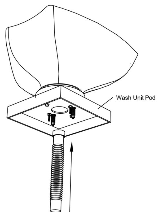
4. Carefully lower basin through cutouts in top of wash point cabinet ensuring basin is pointing forwards. Fix into place using bolts, screws and washers previously removed in stage 2.
